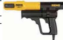
Supplied in carrying case, Electro-hydraulic drive with proven universal motor 230 V or 110 V, 50–60Hz, 450 W. For dimensions 16 - 75mm, turnable pressing jaw entry. Weight of the machine approx. 4,5 kg.
